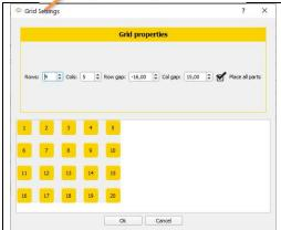
Grid settings dialog appears only if corresponding feeder type selected. Adjust Row / column count to define array dimensions. Row gap and column gap defines pocket distances.
